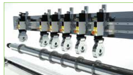
Pneumatic Knife System (Auto. / Manual set up)
